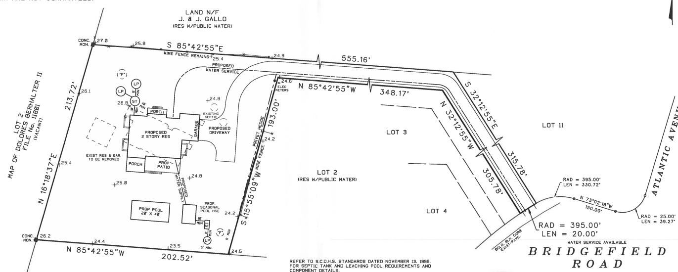
NOTE: SPOT ELEVATIONS RESULT FROM AN ACTUAL FIELD SURVEY AND REFER TO APPROX U.S.C.& G.S. DATUM (M.S.L.).
