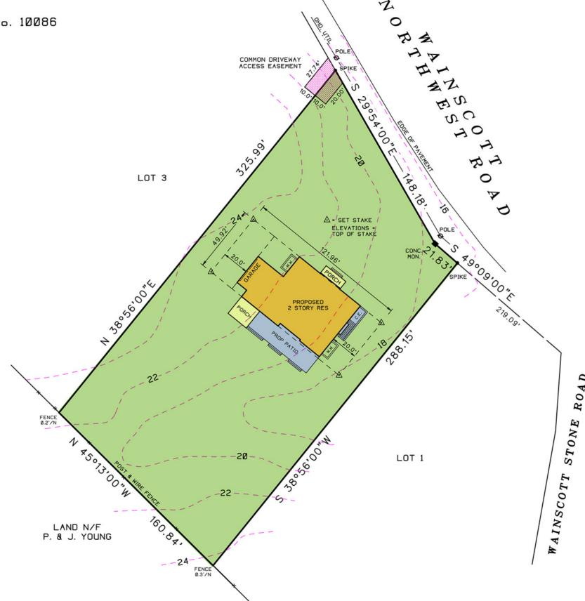
NOTE: TOPOGRAPHIC CONTOURS RESULT FROM AN ACTUAL FIELD SURVEY AND REFER TO U.S.C.& G.S. DATUM (M.S.L.).
